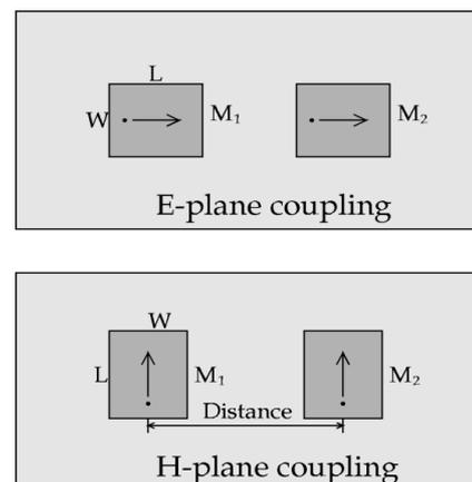
Fig.3. E and H-plane coupled probe fed microstrip antennas.
